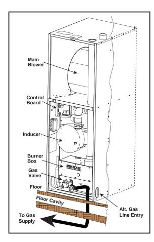
Figure 22. Typical Gas Piping
